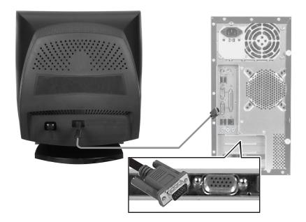
**3** Tighten the screws on the video cable connectors to keep them from coming loose. Tightening the screws also prevents radio and TV interference.
